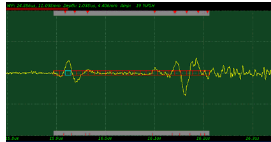
Figure 1: A-scan from the lidded flip chip sample, showing the existing TAMI™ gate setup (26 gates)
