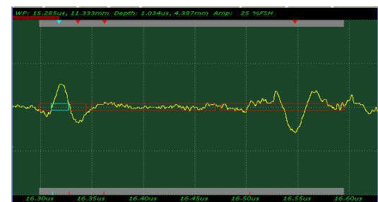
Figure 2: A-scan from the lidded flip chip sample, showing the Flexible TAMI™ gate setup (5 gates)
